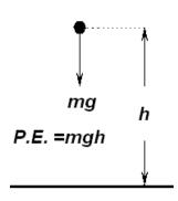
The gravitational potential energy is equivalent to the negative of the amount of work done by the weight of the body in causing the descent. If a mass m is at a height h above a lower level, the P.E. possessed by the mass is (mg) (h) Since h is the height of an object above a specific level, an object below the specified level has negative potential energy
