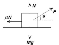
The forces acting on the block as shown in figure Force F will resolve as Fsin $\theta$  along normal while Fcos $\theta$  will be opposite to friction.
